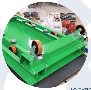
Eccleston Engineering designed a carriage which engaged with elevated tracks and could also act as a stand-alone trolley when fully retracted. Retraction from the nested position saw the casters bear onto newly installed tracks, whilst ground bearing casters allowed for a smooth transition when removing the carriage entirely. A bespoke bump-stop was designed to contain the carriage in normal use and allow for full extraction when necessary.
