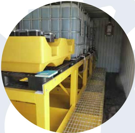
Eccleston Engineering designed a modular system which enabled the process station to be assembled in the container. A robust steel frame with nylon wear surfaces supported and transferred the IBCs through the process, whilst a self-balancing steel containment sump mitigated against any spillages.
